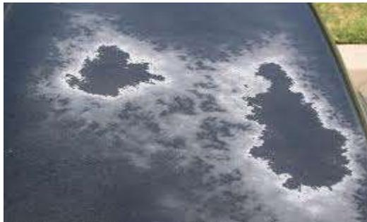
This is what happens when a car has been washed incorrectly or the paint work has not been finished to the right standard.
